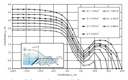
Fig. 2 . Dimensional curves of the free water surface on the permeable sill
