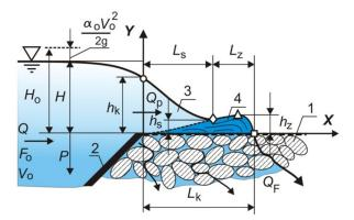
**Fig. 1.** Overflow stream of permeable sill: 1 – stone permeable sill, 2 – sharp-crested weir on upstream slope, 3 – free flow zone, 4 – wave intake (inlet) zone
