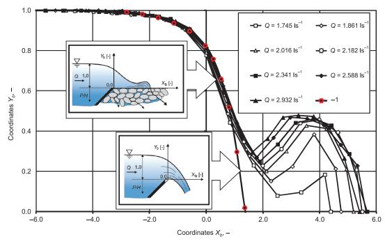
**Fig. 3.** Dimensionless curves of the free water surface on the permeable sill (own research): Q – according to own research, 1 – according to Khan & Steffler (1996) for sharp-crested weir
