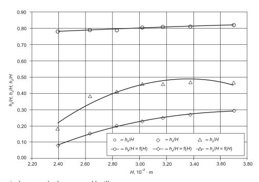
Fig. 4. Dimensionless water depths on permeable sill
